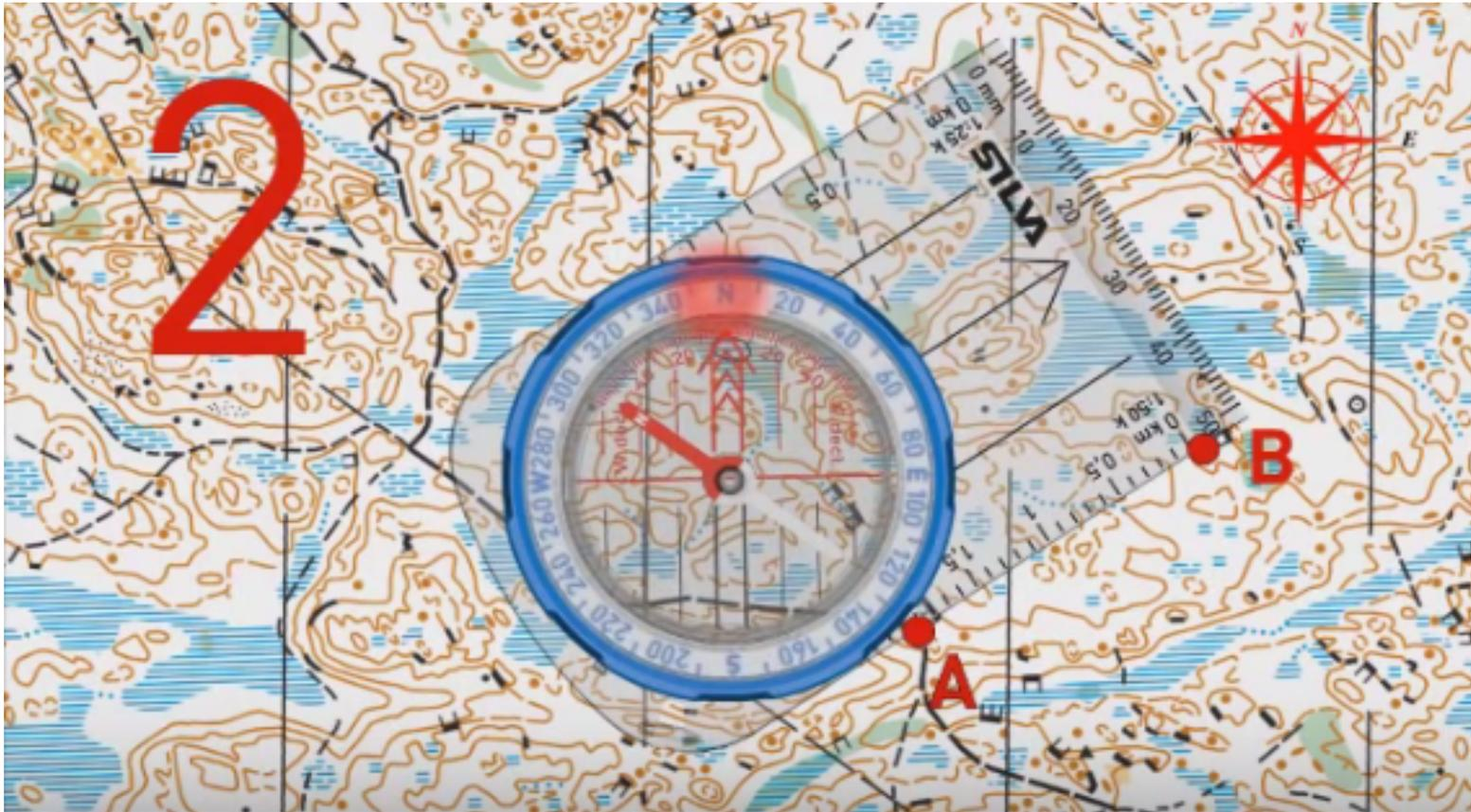
2. Rotate the dial so that the inner lines are parallel with the (North – South) gridlines on the map
